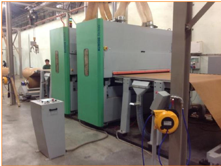
working width 2200 mm (87"), tolerance +/- 0,02 mm (2/2500")
